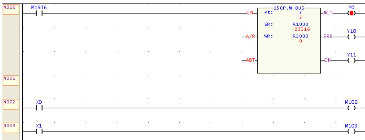
2. Register addresses to be read or written are set in the Modbus Master table; for the register addresses of the slave please refer to 【1.5.1 Application interface contents and Modbus comparison table】.
